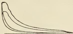
INDICATOR DIAGRAMS FROM 200-HORSEPOWER ENGINE
